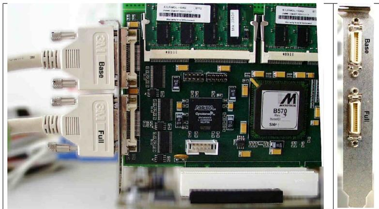
Connect your Camera Link® cable to connect the connector on your camera to the appropriate connector on the frame grabber. Please take attention to connect the Base connector on your camera to the Base connector on the frame grabber. Check the same for the Medium/Full connector.
