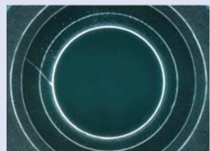
CD Inner Circumferential Scratch
