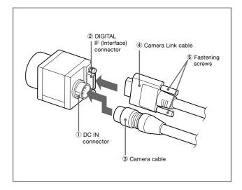
Connect the Camera cable to the DC IN connector and the Camera Link cable to the DIGITAL IF (Interface) connector respectively. When you connect the Camera Link cable, turn the two Fastening screws on the connector to secure the cable tightly.
