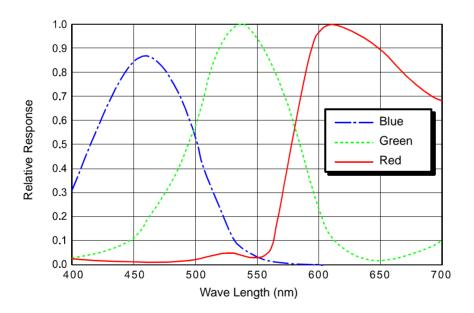
Fig. 14: scA1000-20fc and scA1000-30fc Spectral Response
