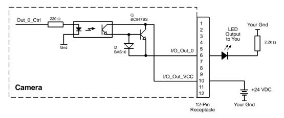
Fig. 40: Typical LED Output Signal at +24 VDC for the External Circuit (Example)
