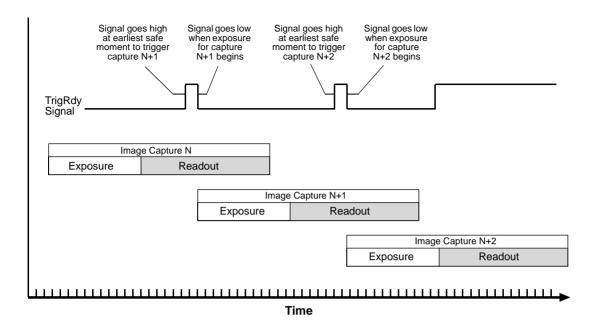
Fig. 50: Trigger Ready Signal
