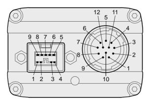
Fig. 36: Pin Numbering for the IEEE 1394b Socket and the 12-pin Receptacle
