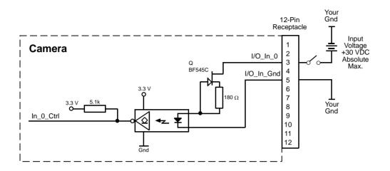
Fig. 38: Typical Input Circuit
