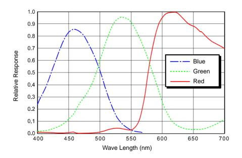
Fig. 18: scA1600-14fc Spectral Response
