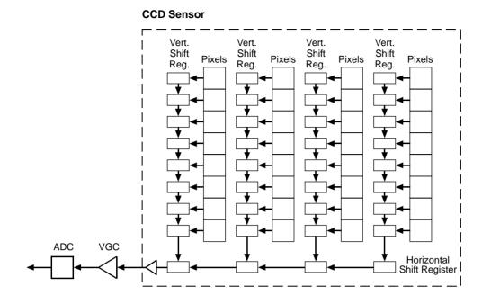
Fig. 31: CCD Sensor Architecture
