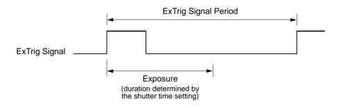
Fig. 44: Programmable Exposure with Rising Edge Activation
