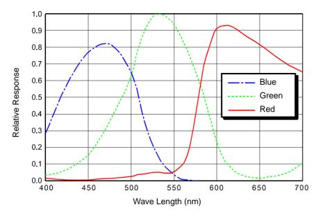
Fig. 13: scA780-54fc Spectral Response
