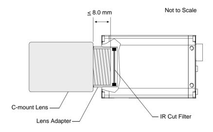
Fig. 25: Maximum Lens Thread Length on Color Cameras
