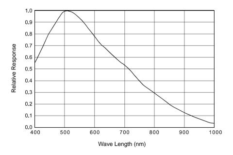
Fig. 5: scA1000-20fm and scA1000-30fm Spectral Response
