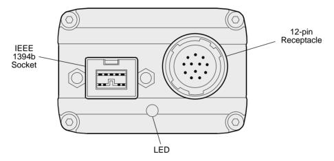
Fig. 35: Camera Connectors and LED
