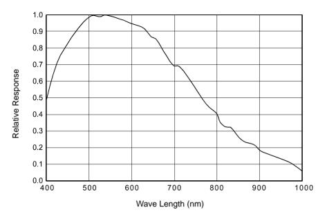
Fig. 8: scA1400-17fm and scA1400-30fm Spectral Response
