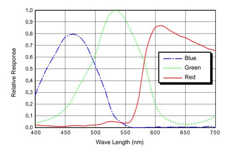
Fig. 10: scA640-70fc Spectral Response
