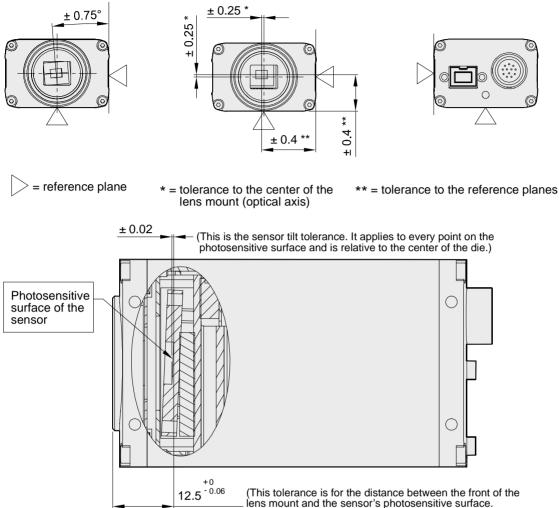
(This tolerance is for the distance between the front of the lens mount and the sensor's photosensitive surface. Note that this tolerance and the sensor tilt tolerance (see above) must be combined to obtain the total tolerance for every point on the photosensitive surface.)
