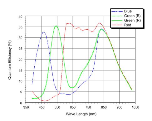
Fig. 12: scA750-60fc Spectral Response
