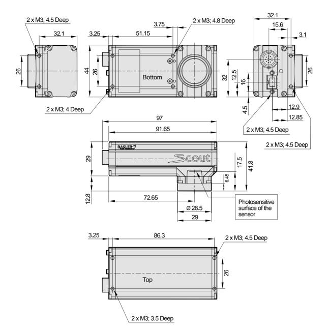
Fig. 23: Mechanical Dimensions (in mm) for Cameras (90° Head) with the Standard C-mount Lens Adapter
