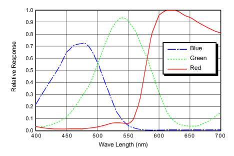
Fig. 17: scA1400-17 fc and scA1400-30 fc Spectral Response
