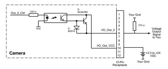
Fig. 39: Typical Voltage Output Circuit
