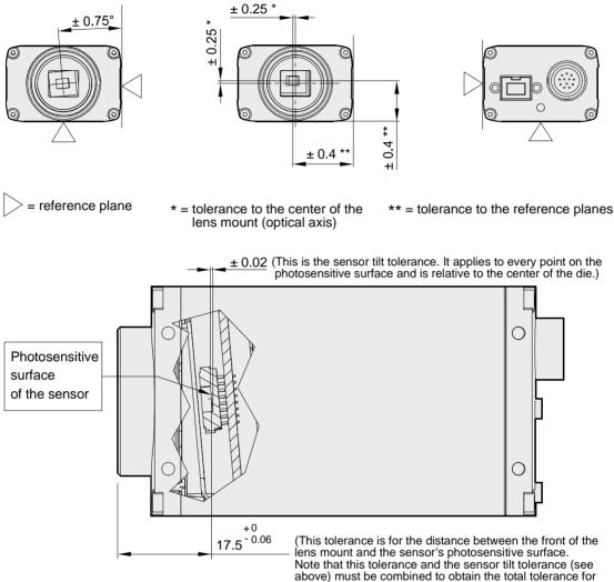
above) must be combined to obtain the total tolera every point on the photosensitive surface.)
