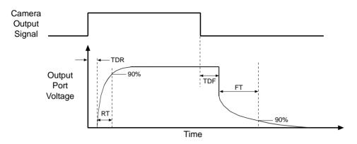
Fig. 41: Output Port Response Times
