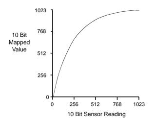
Fig. 67: Lookup Table with Values Mapped for Higher Camera Output at Low Sensor Readings
