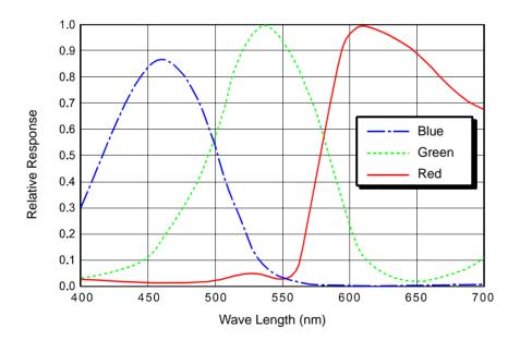
Fig. 16: scA1390-17fc Spectral Response
