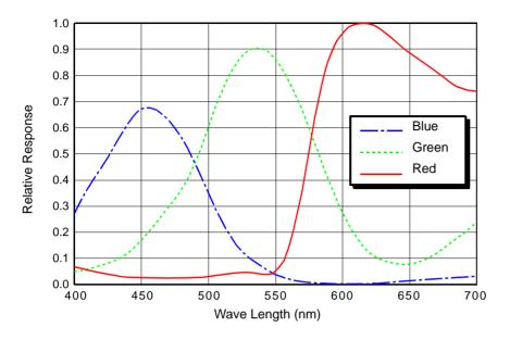
Fig. 15: scA1300-32fc Spectral Response
