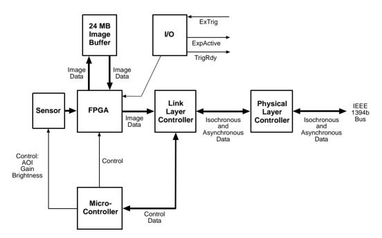
Fig. 34: Camera Block Diagram
