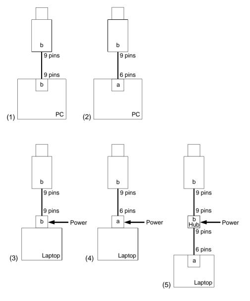
Fig. 26: Different Examples for Linking the IEEE 1394b Compliant Camera to a Computer
