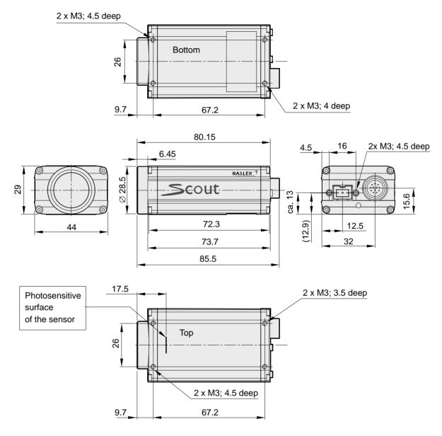
Fig. 19: Mechanical Dimensions (in mm) for Cameras with the Standard C-mount Lens Adapter
