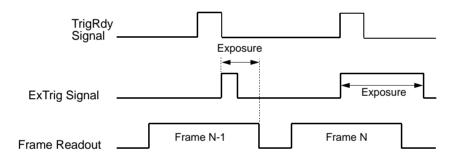
Fig. 46: Overlapped Level Controlled Exposure
