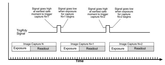
Fig. 51: Trigger Ready Signal
