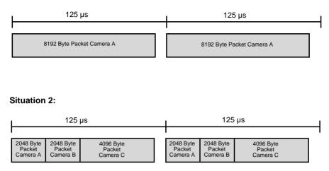
Fig. 72: Packet Transmission During Bus Cycles
