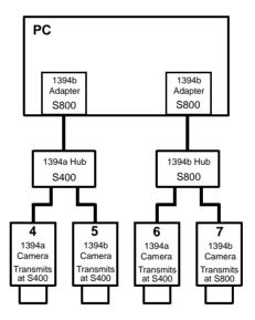
Fig. 73: Examples of Mixed Device Types
