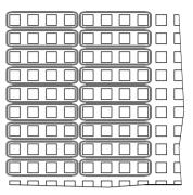
You can combine vertical and horizontal binning. This, however, may cause objects to appear distorted in the image. For more information on possible image distortion due to combined vertical and horizontal binning, see below.
