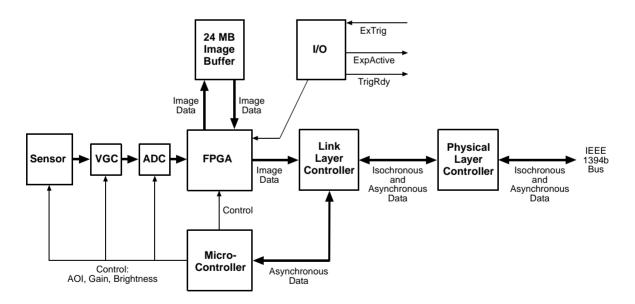
Fig. 32: Camera Block Diagram
