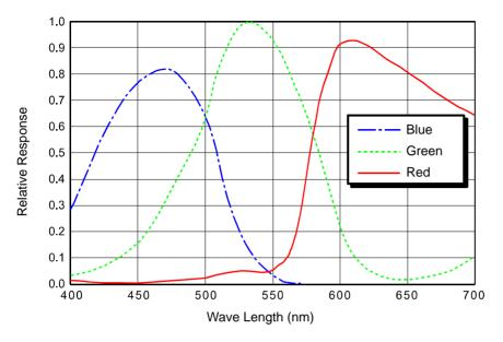
Fig. 11: scA640-74fc Spectral Response
