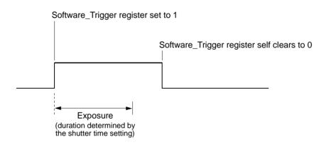
Fig. 43: Programmable Exposure with a Software Trigger
