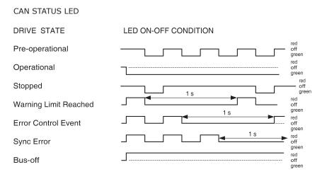
Note: Red & green led on-times do not overlap. LED color may be red, green, off, or flashing of either color.
