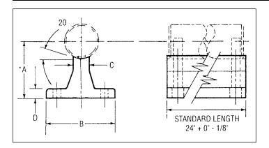
These rails are supplied without mounting holes and can be used horizontally or vertically to provide optimum rigidity (see pre-drilled aluminum rails for sizes and specifications). Shaft support rails are available in standard lengths of 24"+0", -1/8 (600+0, -3.2 mm), but can be supplied to meet shorter length requirements or placed end to end to meet longer length requirements.
