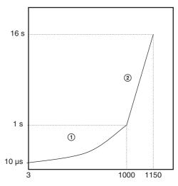
When Auto Shutter is selected, the exposure time is adjusted automatically, based on the brightness of the subject. At this time, the reference level (target point) is set in the AutoExposure register.
