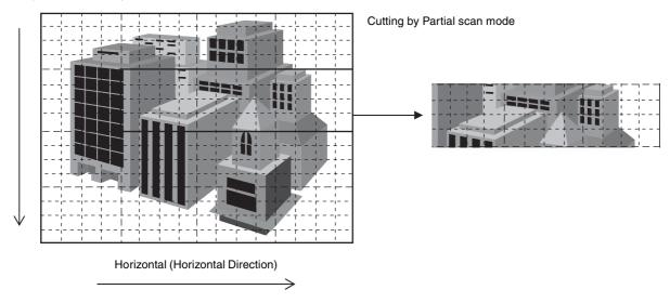
The minimum unit size for partial scan is 32 pixels  $\times$  24 lines. The cut-out position can be set in unit of 4 pixels  $\times$  4 lines. For high-speed scanning, set the maximum packet size.
