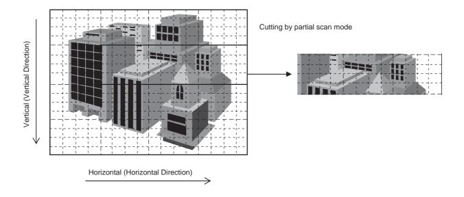
The unit size of both the XCD-SX910CR/SX910UV/SX910 and the XCD-X710CR/X710 is 1/256th of the whole screen, divided into 16 sections, horizontally and vertically.
