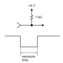
The LOW period that is given by an output wave form is an approximate guideline. It does not correspond exactly to the actual exposure time.
