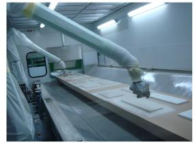
The use of multiple guns both in separate or contemporary allows to reduce cycle times and to use more colors, without having to wash the tubes.
