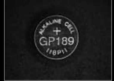
Illumination Low angle LED P.55
